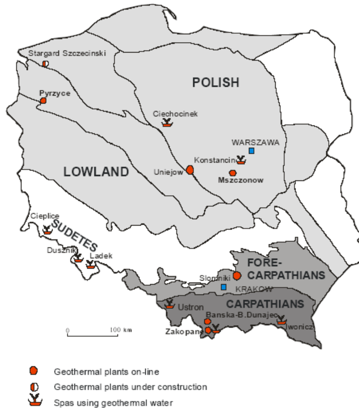
Figure 1. Poland, 2004: geothermal plants in operation, under construction and spas using geothermal waters (division into geothermal provinces after Sokolowski, 1993).
